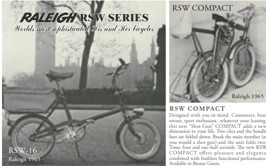
RSW-16 Designed as a convenient adjunct modern living, the new Raleigh RSW-16 provides a perfect form of transport for easy commuting, shopping and moving quickly through traffic, 3-speed Sturmey-Archer gear with twist-grip control, wide profile tires to cushion bumps, quick-release lever-adjusting saddle and control bar stems to fit any height, warper mudguards, fully sprung saddle with thick foam overlay and large capacity detachable carrier bag. The RSW Deluxe incorporates Dynamo-hub built-in generator. Both models available in Beazee Green and Flamingo Red.
